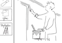
The sensitive parts of the wall need to be glued: wall, door frame/top and bottom edges.
