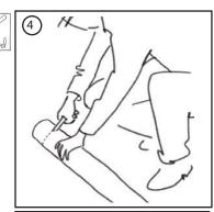
Cut the chuck to the height of the image, using a saw or a cutter. Rewrap it tightly enough on thechuck, before laying it down. (printed side inside).
