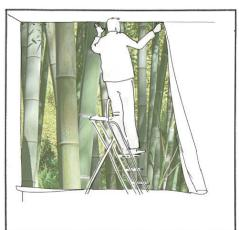
Start hanging your one-piece poster by attaching it to the left corner. Hang it again in the center, with a pin or adhesive strip, then on the far right. Finally, make sure to fix the entire one-piece wall paper every 30 cm.
