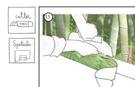
Cut off the excess with a cutter using the spatula (be sure to use a new blade).
