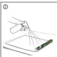
Spray the entire pre-glued surface of the substrate with water.
